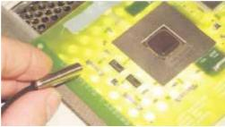
Figure 2. Flexible endoscope under a tape ball grid array.
